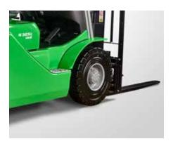
A low step height, large assist grip and wide foot space allow easy access to the operator compartment.
